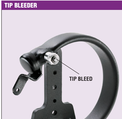
These bleeders allow trapped air to be removed from the bourdon tube. They can also be used for back-flushing or cleaning the system. The tip bleed is available with 316 stainless steel systems. It is accessible by removing the pressure relief back. Tip bleeders are available to 23,000 psi. The capillary bleeder provides an external case connection to the internals
